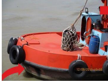
Secured equipment by net prior lifting
