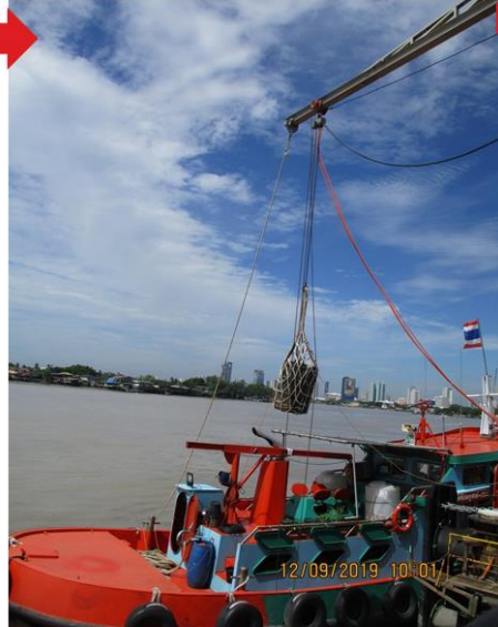
Lifted equipment by jetty pneumatic hoist which is capacity 2 tons
